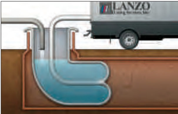
figure1: Direct inversion installation per ASTM F1216
