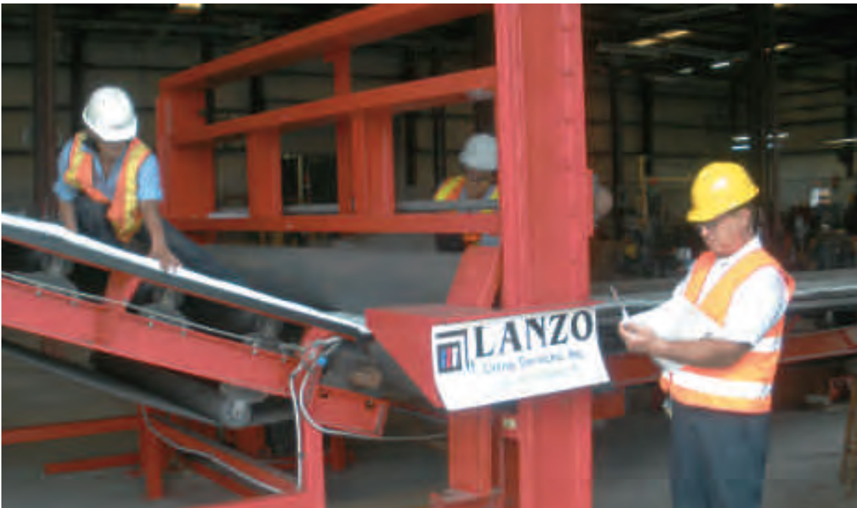
Quality controlled tube impregnation at one of Lanzo Lining Services' state of the art wet out facilities
